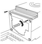
Set the machine upright and remove the two remaining bolts from the back.
